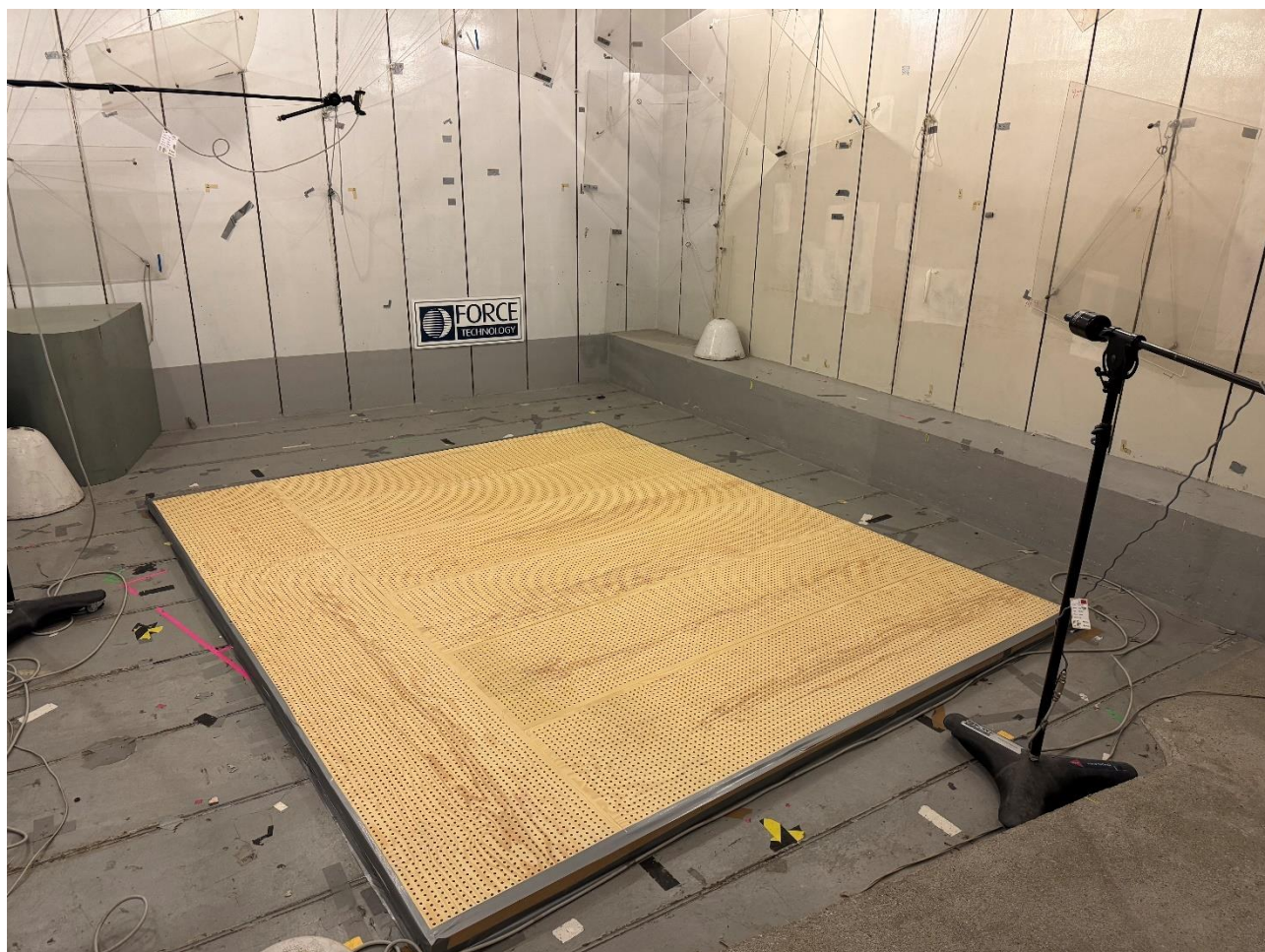
Figur 4 Foto af Keflico Keflico Design Panels SONO, Ø8/cc32mm monteret i laboratoriet.
