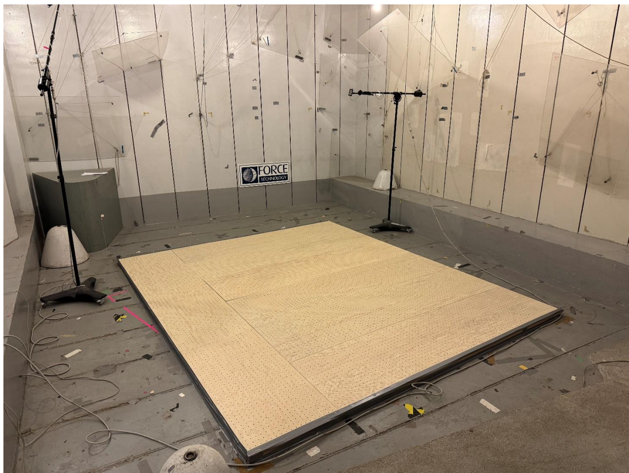
Figur 1 Foto af Keflico Keflico Design Panels SONO, Ø6/cc32mm monteret i laboratoriet.
